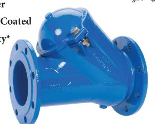
Recommend minimum flow velocities of 2<sup>ft</sup>/sec. Horizontal installation requires approx 20<sup>ft</sup> of static head for positive sealing.
